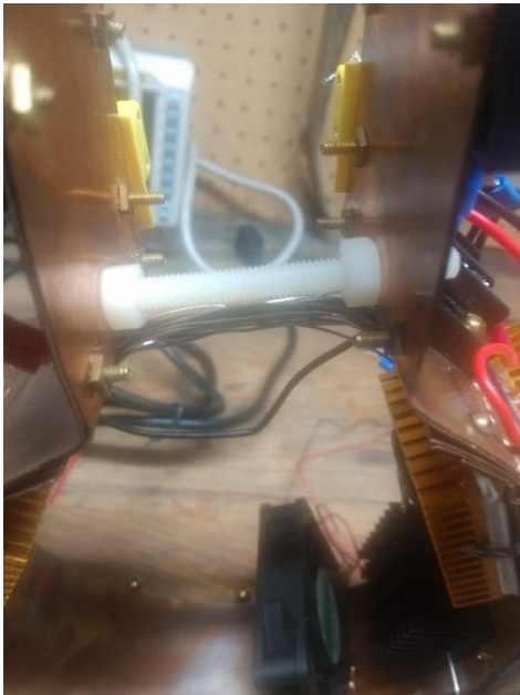
Figure 4. Ring Gap Detail – Adjustable gap distance with Constantan wire thermocouples mechanically connected to the ring. Non-conductive bolt/nuts adjust the gap and stabilize the ring.
