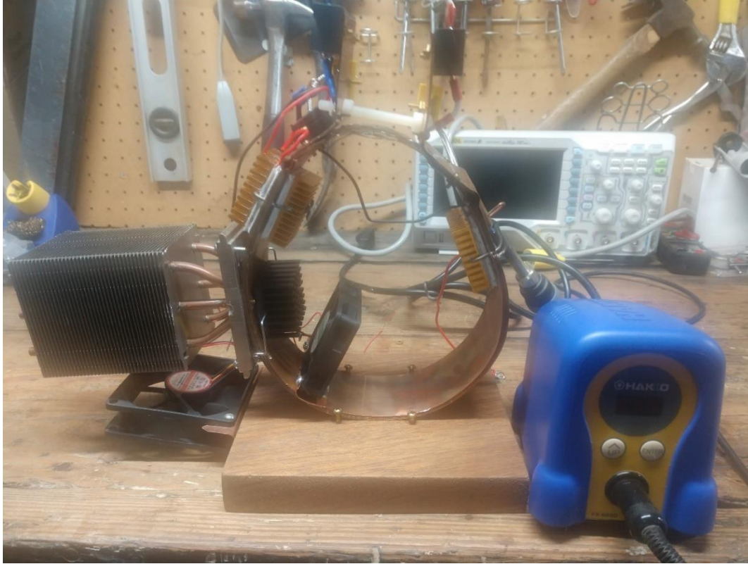
Figure 1. Front View – cooling system on the left, heating system on the right. Note: I may try to get this to look more like a ring, but it is hard to do that and maintain the flat surfaces to mount the TEC's and heat sinks.
