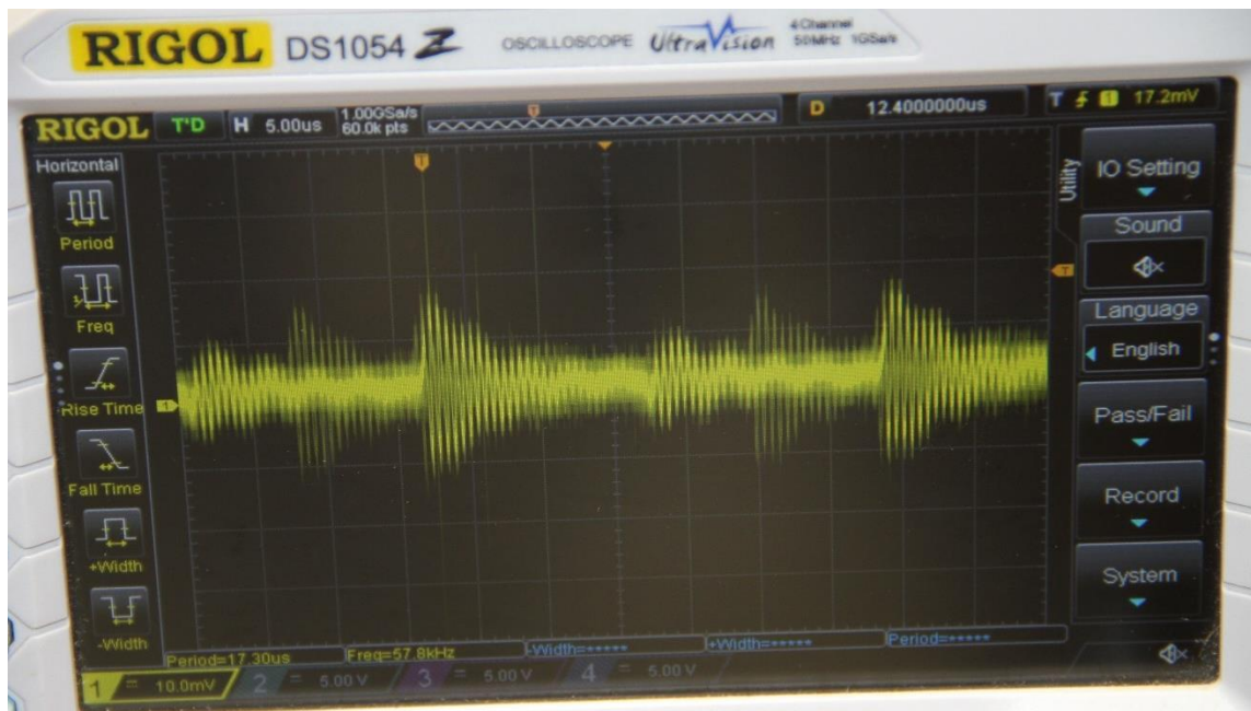
Figure R3. Scope Ring Gap Voltage Output with Ring Power Off (57.8kHz, 30mVolts peak-to-peak). See the video for output when the ring is operating.
