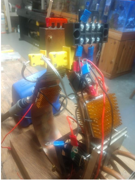
Figure 3. Cooling Side – Active cooling near gap: 2 TEC's on both sides of the ring, Passive cooling: Large capacity heat sink with fans to intercept heat from hot side of ring. Also has a thermocouple to measure temperature or provide an additional voltage source.
